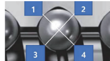
Fig.1.1.3 Single Nut with four-point contact
